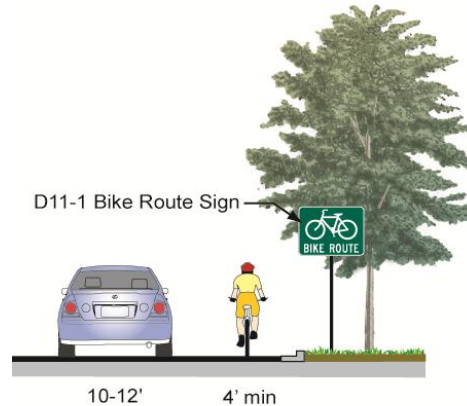
Bike Route with Wide Shoulder and Bicycle Friendly Rumble Strip
