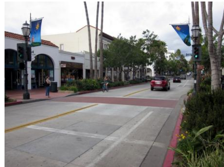
Mid-Block Pedestrian Signal
