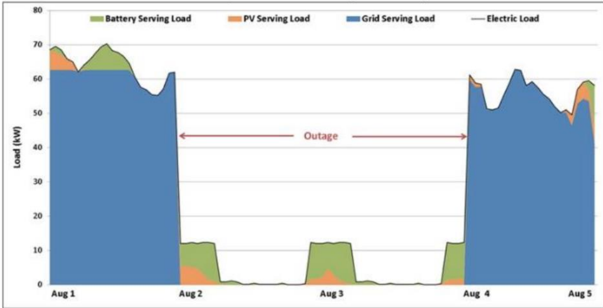
Solar+Storage Providing Backup to Critical Load During Grid Outage Events
