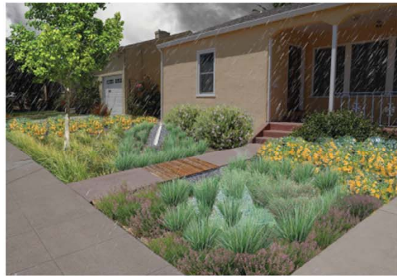
▲ RETROFIT OPPORTUNITY: The same residential yard that converts un-watered grass areas into a rain garden with drought-tolerant landscaping. Roof downspouts direct water into the rain garden and a bridge connects the spaces.
