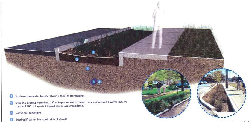
Cutaway view of a bioretention swale. Stormwater would flow into the swale and infiltrate into a layer of fast-draining bioretention soil, and the underlying soils. Where feasible, an underdrain below the bioretention soil would allow treated water to enter the storm drain system.
