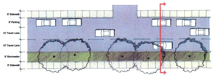
**Concept:** Alternating Stormwater Swales and Parking Zones
