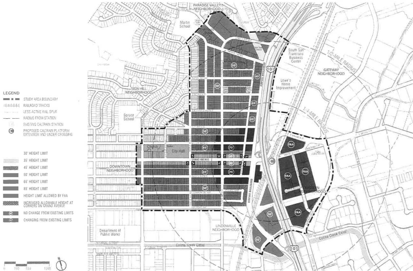
Figure 5.02: Allowable Building Heights
