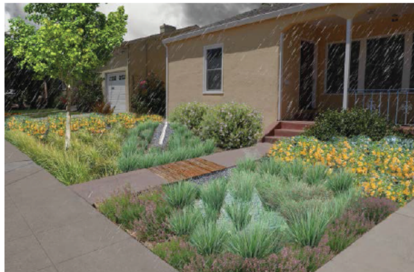
▲ RETROFIT OPPORTUNITY: The same residential yard that converts un-watered grass areas into a rain garden with drought-tolerant landscaping. Roof downspouts direct water into the rain garden and a bridge connects the spaces.
