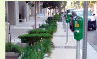
▲ Streets with on-street parking should have paved step out zones and frequent perpendicular access points to the sidewalk zone between planters.
