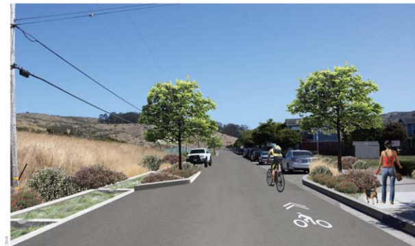
▲ RETROFIT OPPORTUNITY: The same street with a combination of a vegetated swale and stormwater curb extensions.
