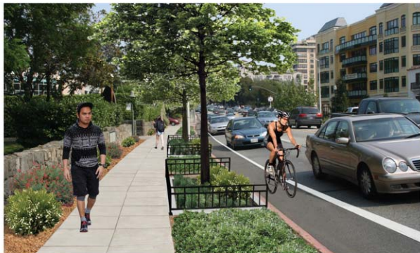
▲ RETROFIT OPPORTUNITY: The same commercial street with tree wells to capture and treat stormwater runoff and bike lanes to define space for cyclists.
