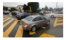
could help improve driver behaviors, preclude vehicles from blocking the intersection, and improve pedestrian safety dramatically. This could be an ideal location for a mini-circle, or at very least creating barriers on the curb extensions so that vehicles can not cut across the curbs.
