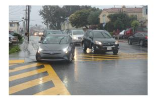
• **Barriers on the curb extensions.** First include some type of planter, vertical delineator, or other barrier to preclude vehicles from driving over the curb extensions, especially the one on the southwest corner. This is exceptionally dangerous to pedestrians, and unsafe for vehicles as well.
