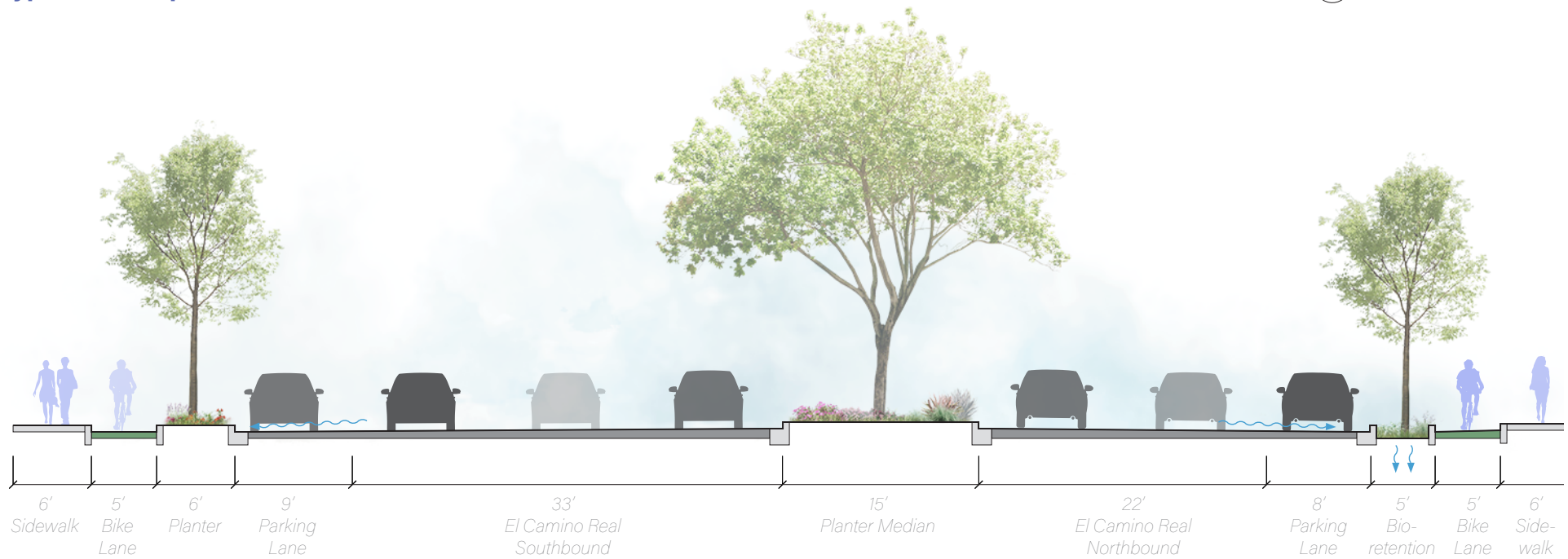
Typical Cross Section Detail: El Camino Real
