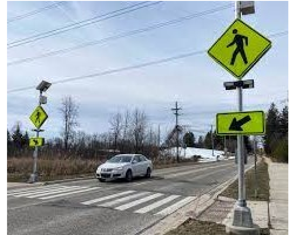
Rectangular Rapid Flashing Beacon (RRFB's)
