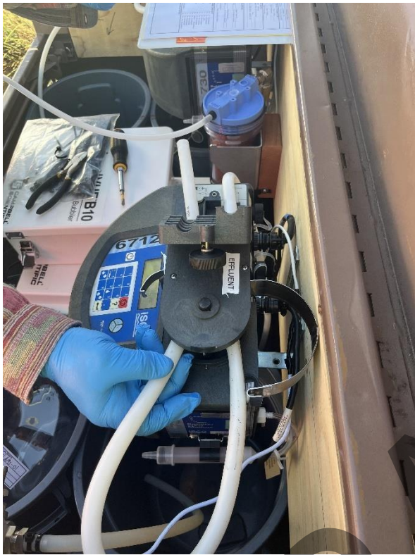
Figure 2. Peristaltic SEB (styrene ethylene butylene styrene) pump tubing that is replaced prior to each sampling event and prior to the field blank sampling.
