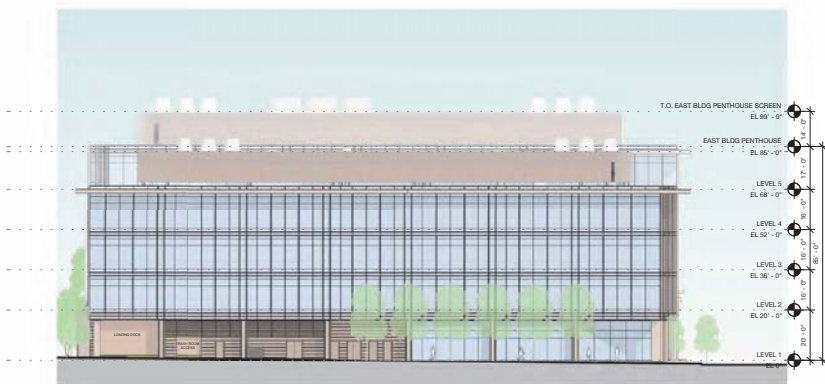
2 OLD COUNTY ROAD (WEST) OVERALL ELEVATION 1" = 20'-0"
