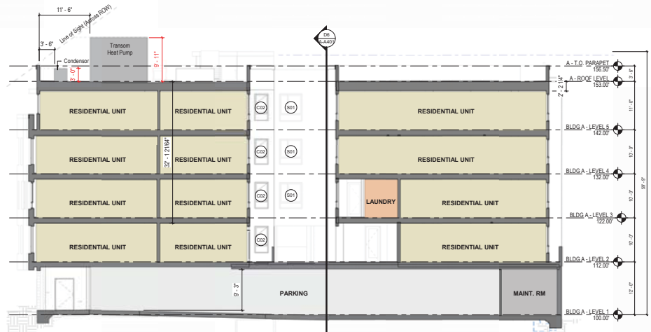
A4 BLDG A - SECTION - NORTH FACING 1/8" = 1'-0"
