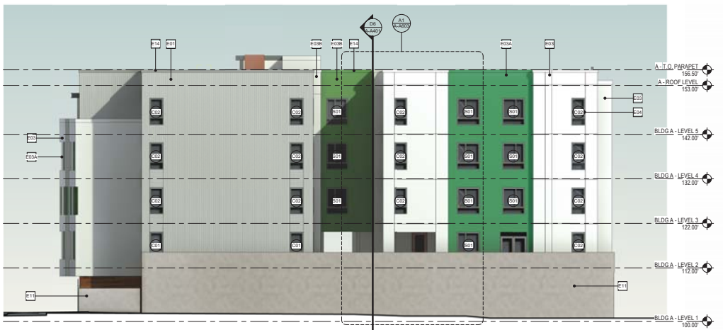
A1 BLDG A - SOUTH-WEST ELEVATION (BACK) 1/8" = 1'-0"
