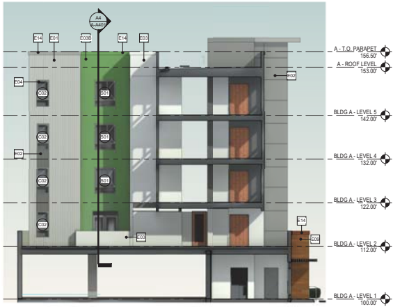
D1 BLDG A - COURTYARD ELEVATION 1 1/8" = 1'-0"
